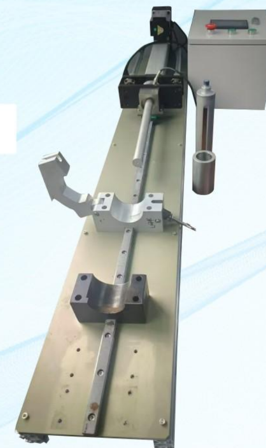
发电机线包电控装卸工装 Alternator coil pack electrical assembly and disassembly tooling
